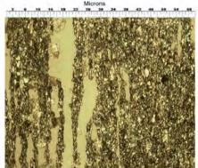
500x Ferrous wear debris and dust/dirt.
